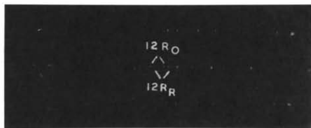
Fig. 4. a -axis 15^\circ oscillation photograph of a dendritic single crystal, showing reflections of 12R_R and 12R_O (one reflection for each polytype is marked by an arrow), camera radius 3 cm; Cu K\alpha radiation.
